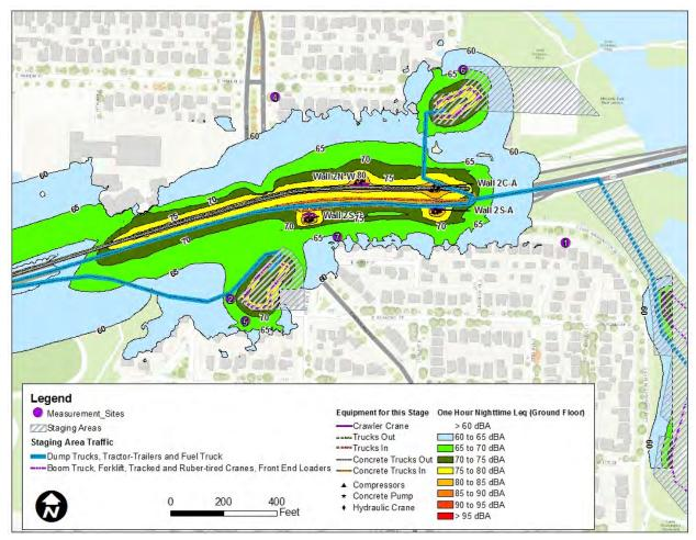
Nighttime modeled noise levels during construction of the North Lid Wall (identified as wall sections 2N-W and 2S-B), and the Center Lid Wall (identified as wall sections 2C-A and 2S-A) using compressors with mitigation would meet the proposed noise level limits at all residential locations. Mitigation requirements for the compressors are described in the required minimum mitigation measures section.
