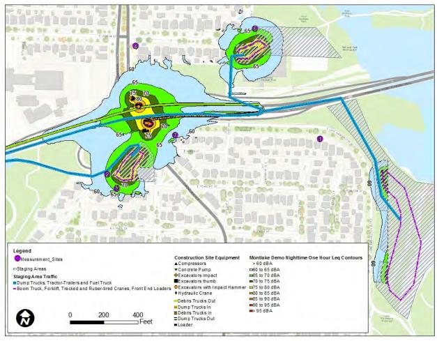
Nighttime modeled noise levels during the demolition of the existing Montlake Boulevard E. structure using compressors with mitigation would meet the proposed noise level limits at all residential locations. Mitigation requirements for the compressors are described in the required minimum mitigation measures section.
