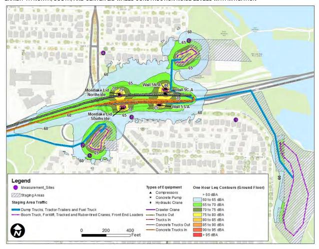
Nighttime modeled noise levels during construction of the North Lid Wall (identified as wall section 5N-A), the Center Lid Wall (identified as wall section 5C-A), and the South Lid Wall (identified as wall section 5S-A) using compressors with mitigation would meet the proposed noise level limits at all residential locations. Mitigation requirements for the compressors are described in the required minimum mitigation measures section.
